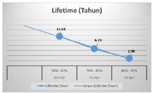
Fig. 1. Relation between loading factor and lifetime.
