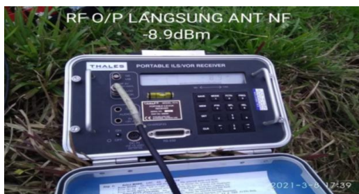
Fig. 6 Results of PIR Measurement on Nearfield Antenna
