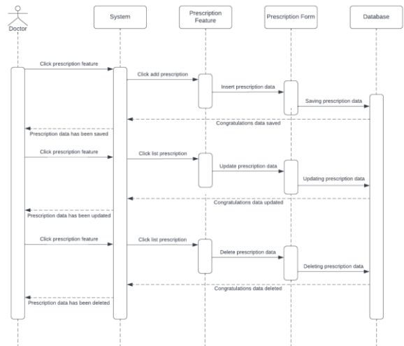
Fig. 6. Sequence Diagram for Manage Prescription Feature
