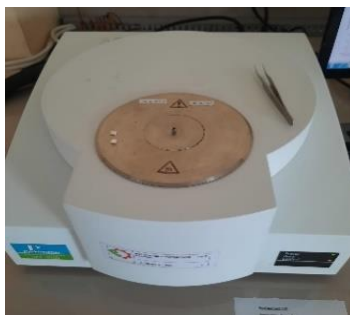
Gambar 2. Differential Scanning Calorimetry
