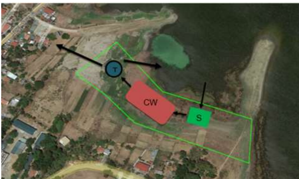
Figure 4. Wastewater flow in Nagbacalan village (S: Screening, T: Tank, CW: Constructed wetland)
