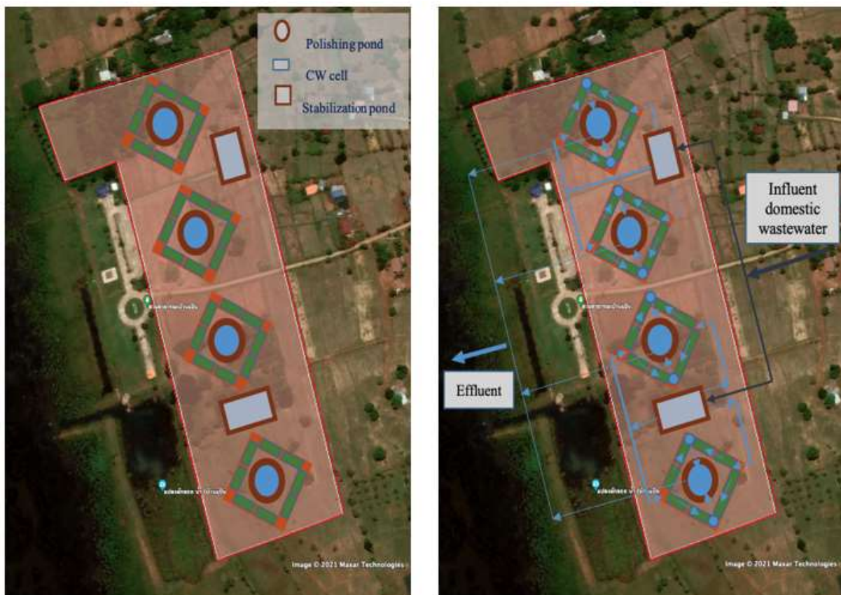
Figure 10. Proposed constructed wetlands and supporting facilities near the Nong Han Lake: (a) location and layout and (b) treatment system flow.
