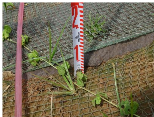
Figure 11. Level difference in the border line between the sheet plot and another similar sheet plot after 3 months
