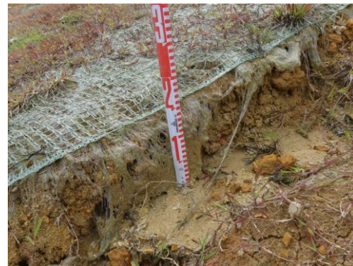
Figure 7. Level difference in the border line between the sheet covered plot and the neighbor bare plot after 13 months
