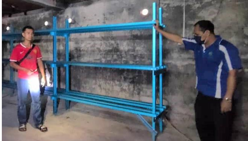
Figure 6: 'C-channel Blue' iron (0.75mm) was Used to Make the Media Bag Placement Rack.
