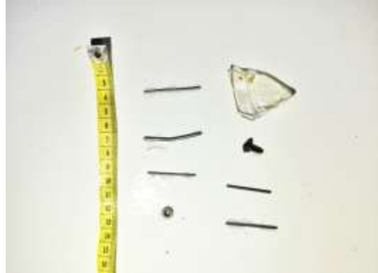
Gambar 2. Benda asing logam ( mur, baut, pecahan kaca, paku).
