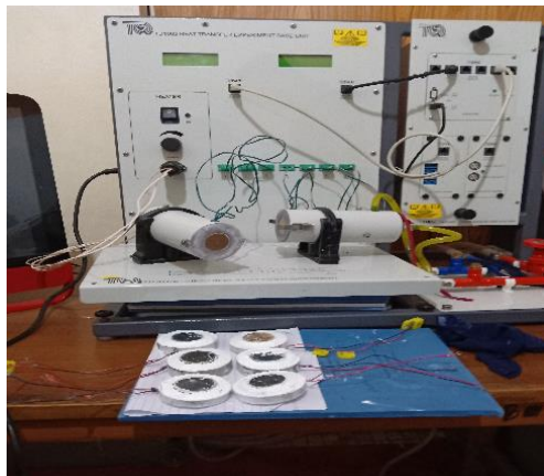
Fig. 6. Thermal conductivity test of composite PCM
