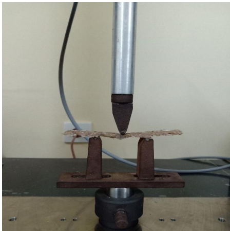
Fig. 4. Bending test of composite PCM
