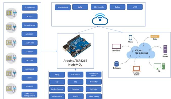
Fig 7. IoT Architecture for Energy Monitoring
