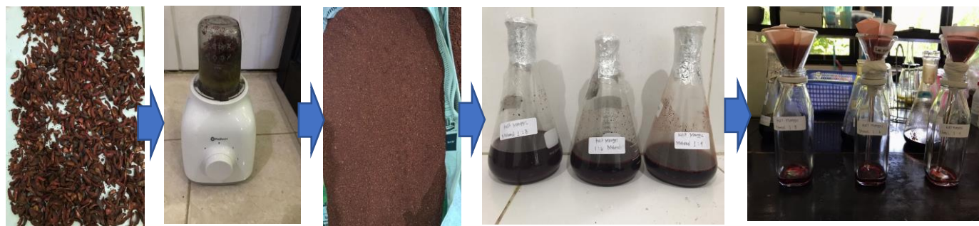
Fig. 2. The process of extracting natural dyes from mangosteen peel waste.
