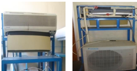
Figure 3. Split AC with ejector system design
