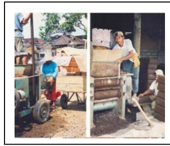
Figure 4 The mill operator push the raw material using their foot or hand
