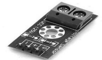
Gambar 7. Sensor tegangan 0-25 V.
