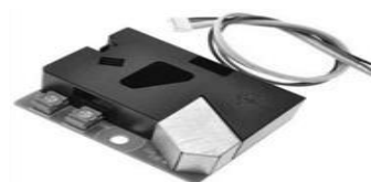
Gambar 9. Sensor debu DSM501A.
