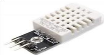
Gambar 8. Sensor suhu DHT22.
