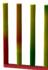
Gambar 10. Simulasi distribusi larutan nutrisi rangkaian vertical.
