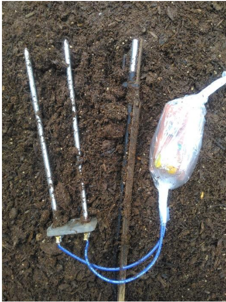
Gambar 12. Sensor DS18B20, probe kadar air dan Oscillator 555
